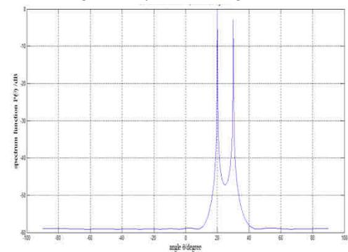
Fig.2: Power spectrum plot (power (dB) v/s angle (degrees)) of improved MUSIC algorithm.
